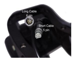
The long **6 pin** cable connects directly to the motor. The motor controller is contained inside the motor housing and a short cable with a matching connector emerges from the housing.
