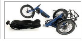
Save space: The Delta tx features a unique split frame design. The only tool you need is an Allen key for the frame connection and the handlebar stem. Find out how to do this in the video on our website www.hpvelotechnik.com
